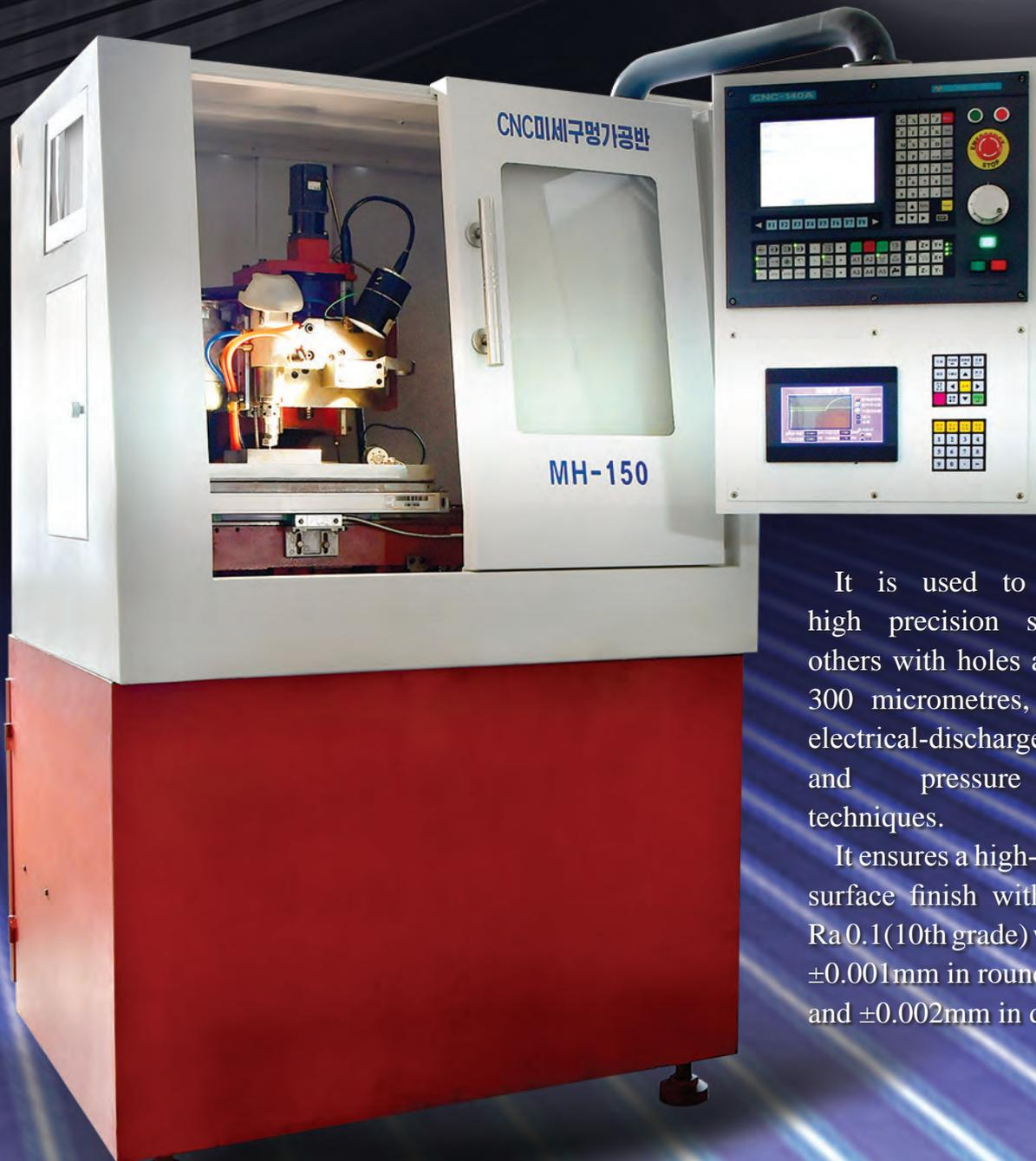
It is used to process with high precision spinnerets and others with holes as small as 80-300 micrometres, based on the electrical-discharge machining and pressure processing techniques.
