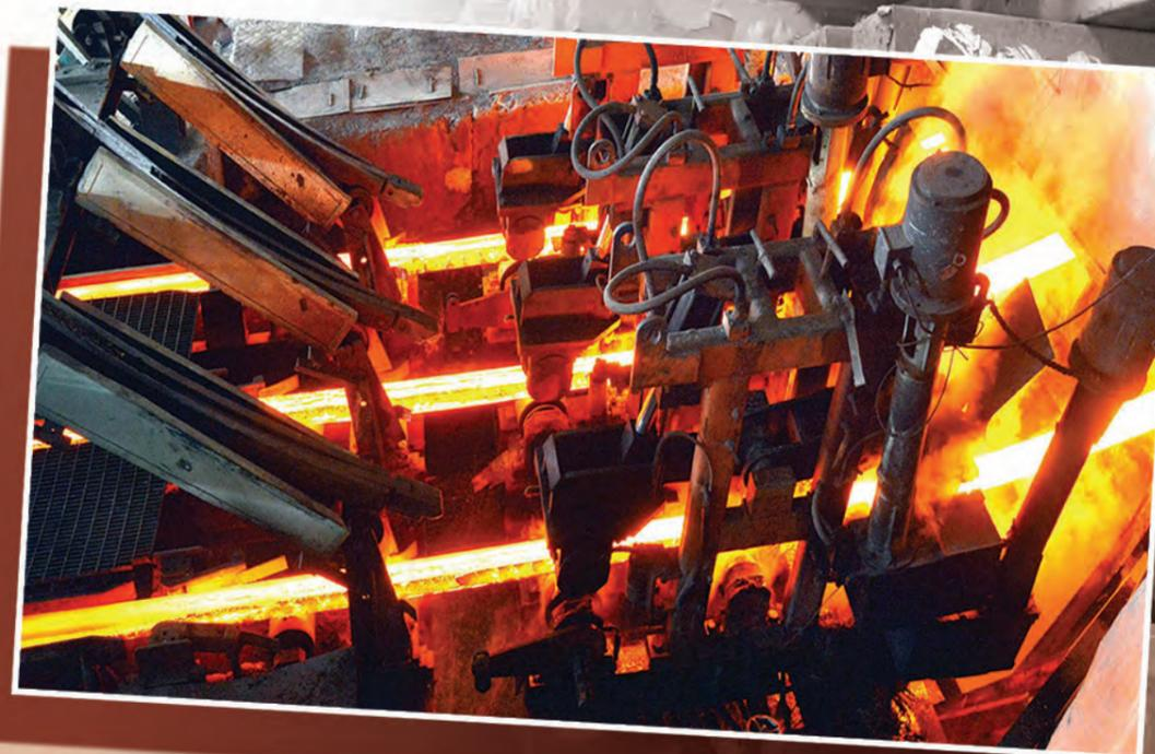
The complex has recently established the steel production process relying on local raw materials and fuel, streamlined the continuous ingot-moulding process and introduced into rolling and other related processes high-temperature air combustion technology based on coal gasification so as to increase rolled steel production.
