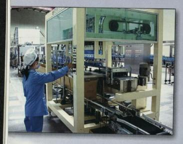
The Kangso Mineral Water Processing Factory specializes in the production of mineral water good for health and longevity. Equipped with automatic facilities throughout the whole production process ranging from 6-stage filtering process to precision filtering and ultraviolet s crilizing, processes, the factory turns out the mineral water filled in PET bottles.
