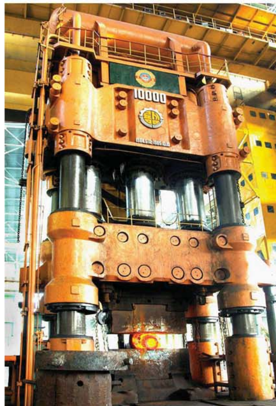
A 10 000-ton press equipped with CNC technology.
