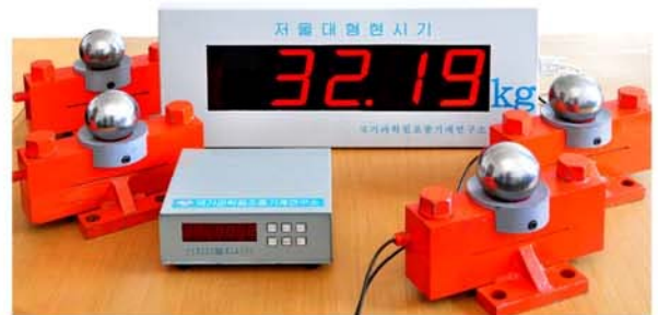
Scales equipped with newly developed weight-sensing elements.
