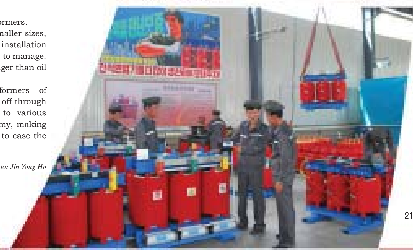
Energy-saving air transformers of different capacities are produced and sent to various sectors of national economy
